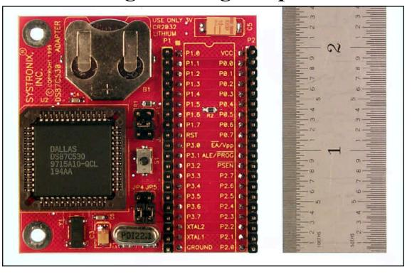
Develop with the new DS87C530 High Speed Microcontroller.
